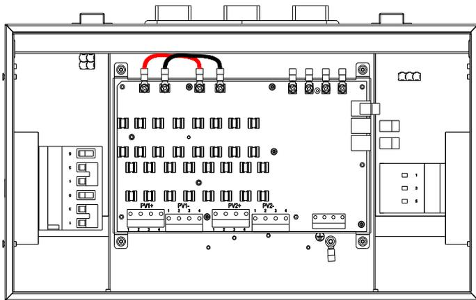
Figure 3-13 Wire connection in the Wiring box (1 MPPT working alone)
