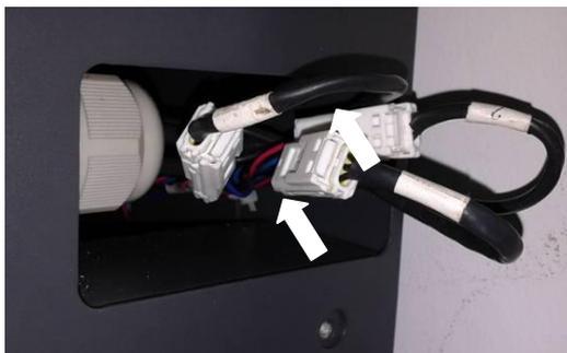
Figure 6-10 Plugging the wire connectors
