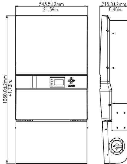
Figure 3-1 Dimensions of CPS SC20KTL-DO/US-480
