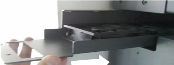
Figure 6-6 Inserting the fan tray assembly
