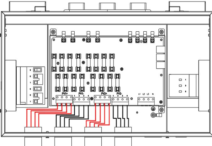
Figure 3-12 Wire connection of DC input
