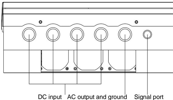
Figure 3-9 Knockouts for cable entry
