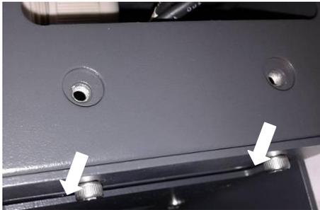
Figure 6-12 Fixing the fan bracket on the right side
