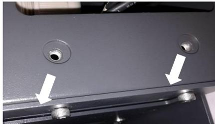
Figure 6-4 Unscrew the fan bracket on the right side
