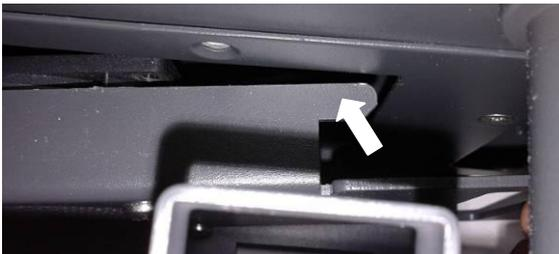
Figure 6-7 Hooking the fan tray assembly
