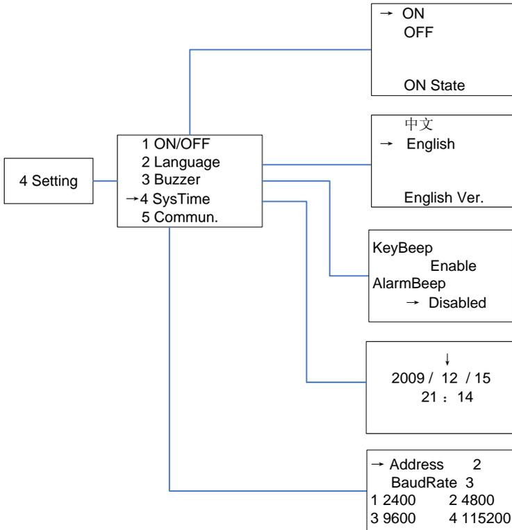
Figure 4-11 System setup menu and submenu
