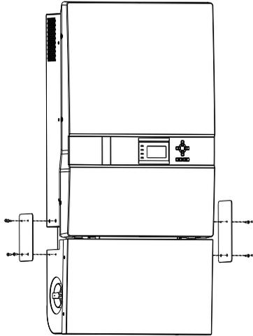
Figure 6-13 Securing panels on both sides
