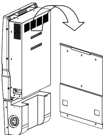
Figure 3-7e Mounting inverter on the bracket
