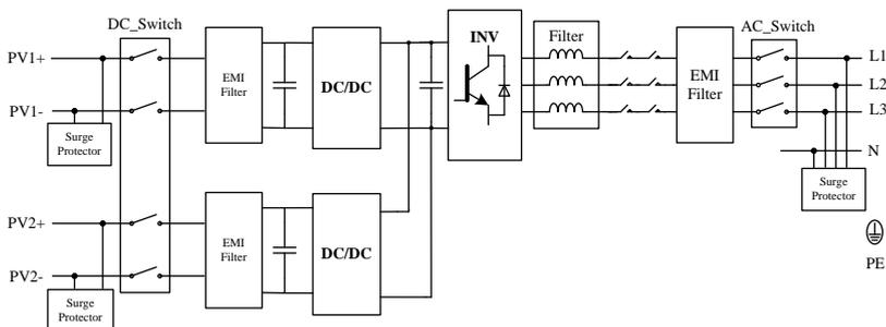
Figure 2-2 Schematic diagram of CPS SC20KTL-DO/US-480
