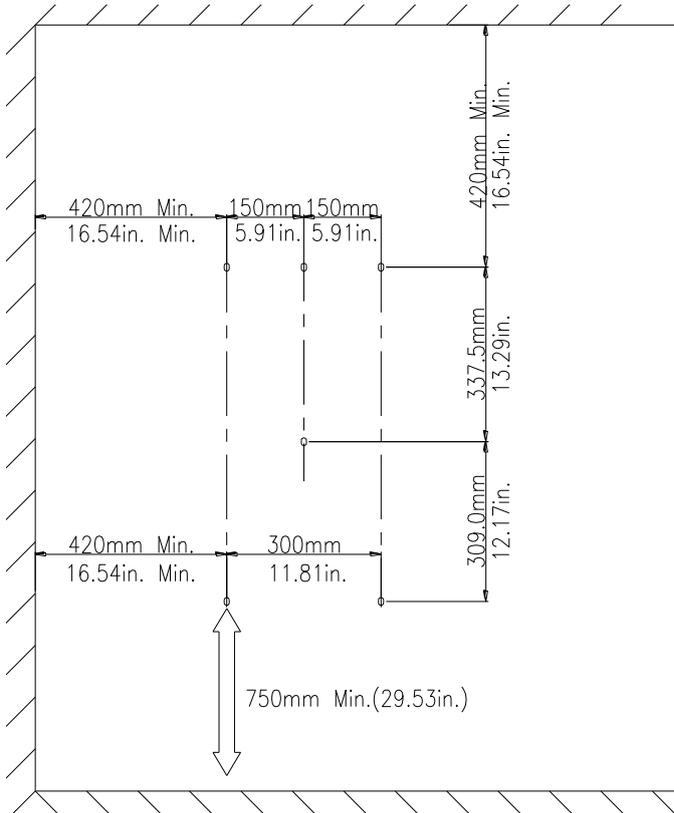
Figure 3-4 Bracket mounting dimensions
