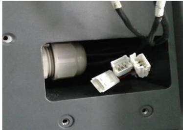
Figure 6-2 Unplugging the wire connectors
