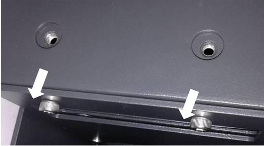
Figure 6-11 Fixing the fan bracket on the left side
