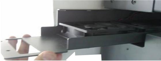
Figure 6-5 Pulling out the fan tray assembly
