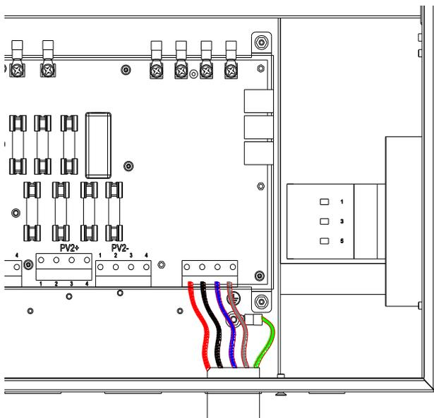
Figure 3-18 Diagram for wire connection of AC output and Grounding
